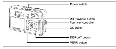
If the Initial Settings screen or Date Adjust screen appears when you turn the camera on, follow the procedure below to set the display language and/or current date and time.
